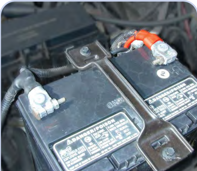
W5E: ACID AND CHEMICAL RESISTANT. USE TO SEAL CABLE/TERMINAL JUNCTIONS.
