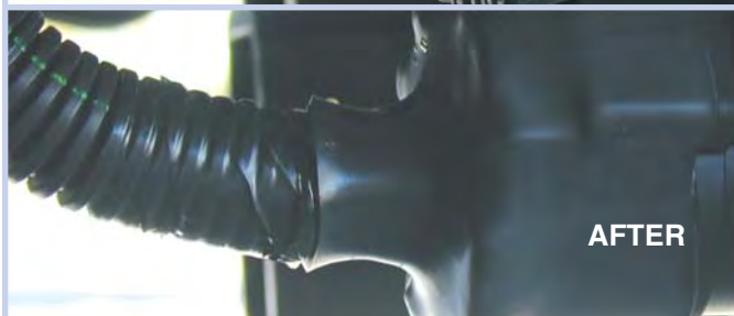
W3B2 (4X): USE FOR STRAIN RELIEF; SLIP OVER A LARGE CONNECTOR AND SHRINK TO SMALL WIRE.
