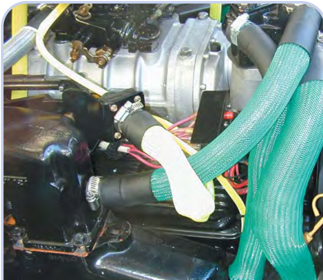
BRAIDED SLEEVING: RESISTS ABRASION AND IMPROVES APPEARANCE. O2B2: SHRINK TO HOLD IN PLACE.
