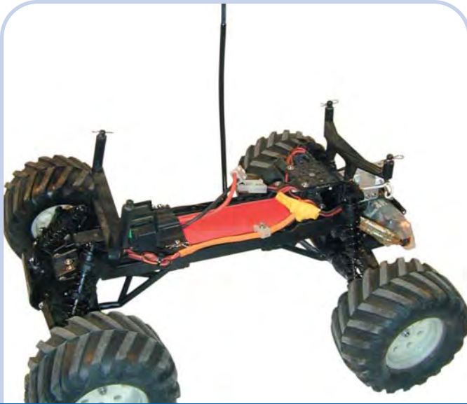
W5DL: LENDS ADDITIONAL SUPPORT TO RC CAR ANTENNA. B2: PROTECT AND COLOR CODE WIRES.
